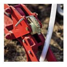
The one-to-one parallel linkage maintains constant opener angle relative to the soil and opener depth relative to the packer wheel throughout its range of travel. The opener can contour up 25 cm (10 inches) and down 18 cm (7 inches).
