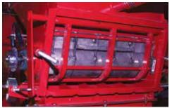
A hydraulic valve manifold providing all operator adjustments is conveniently located on the air cart.
